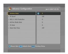
To configure the network environment for the digital receiver in detail, select the Installation > LAN Setting > Advance Configuration menu.
